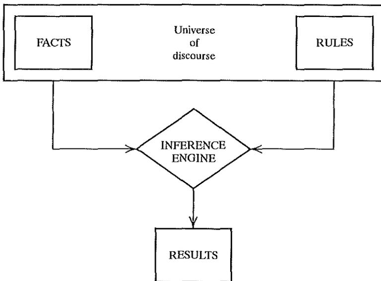
Fig. 3.- The structure of an expert system (After Gardin; 1986, p. 8).
